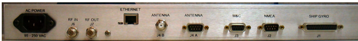
Figure 4-1 Rear Panel DAC-2202 ACU
